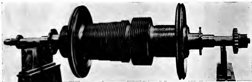
Fig. 6. View of high pressure turbine spindle showing ahead and astern (right) impulse wheels, ahead reaction blading, water gland runners, thrust collar, governor drive gear (left) and flexible coupling (right).
